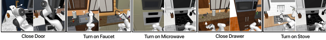
Figure 4: A suite of simulated tasks for benchmarking performance of policy mobilization methods. We pick five single-stage manipulation tasks from the RoboCasa benchmark [19]: (1) Close Door : push or close the microwave or cabinet door using the robot gripper. (2) Turn on Faucet : precisely move the faucet handle to turn on water. (3) Turn on Microwave : push a small button on the microwave. (4) Close Drawer : close an open drawer next to the robot. (5) Turn on Stove : turn a specific knob out of six knobs on the stove. Here, we visualize two successful rollouts for each task. Note that episodes are executed in environments with different layouts and textures. In the Close Door task, the robot might encounter either a cabinet door or a microwave door. The Turn on Faucet , Turn on Microwave , and Turn on Stove tasks require accurate robot placement to be executed correctly. In the Close Drawer task, the drawer can be either on the left or right side of the robot.
