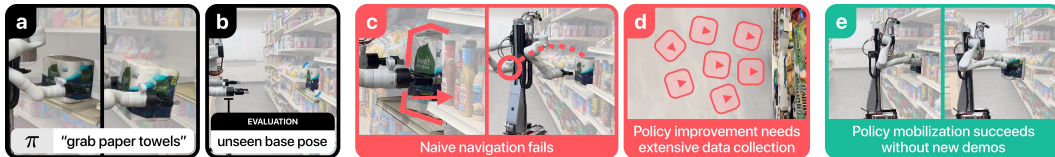
Figure 1: Introducing policy mobilization. (a) Assume a visuomotor policy \pi trained from one or a set of limited camera poses. (b) We are interested in running \pi on a mobile platform, where the robot is initialized at a random pose and needs to navigate before running \pi . (c) Naively navigating towards the object of interest and executing the manipulation policy is likely to result in an out-of-distribution initialization for the policy, leading to failures. Left: The robot gets too close and pushes the object inward with the arm. Right: suboptimal heading makes the object unreachable for the left arm. (d) Improving the robustness of the policy requires extensive data collection to cover all possible robot base pose initializations. (e) We define the new problem of policy mobilization which aims to find the optimal robot pose that leads to an in-distribution viewpoint for executing \pi , achieving task success without the need to collect additional demonstrations.
